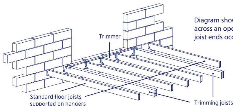
Diagram showing the use of a trimmer across an opening where three or more joist ends occur at the opening.
