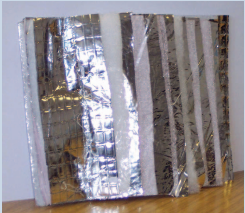
Cut-away picture of a multi-foil insulation material showing the layers
