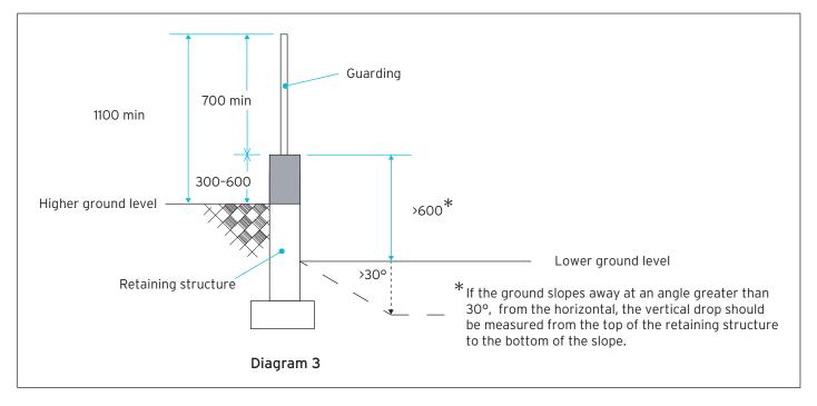
Diagram 3 shows a raised retaining structure which is between 300-600mm above the higher ground level where young children could climb up and stand on the wall and where the drop from the top of the wall to the lower ground level is more than 600mm. In such cases guarding is required and should extend at least 700mm above the top of the wall to protect young children from toppling over the guarding.
