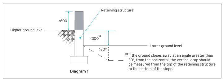
Diagram 1 shows a raised retaining structure which is higher than 600mm above the higher ground level and where the difference in ground levels is less than 300mm and therefore considered to pose a low risk of injury from older children or adults falling over the wall. In such cases guarding is optional.
