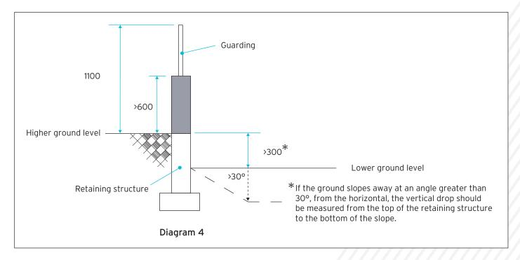
Diagram 4 shows a raised retaining structure which is more than 600mm above the higher ground level together with a difference in ground levels of more than 300mm. The height of the raised section protects against young children climbing and stand on the wall and the guarding protects older children and adults from toppling over the wall and falling more than 900mm.
