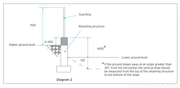
Diagram 2 shows a raised retaining structure which is between 0-300mm above the higher ground level where young children could climb up and stand on the wall and where the drop from the top of the wall to the lower ground level is more than 600mm. In such cases guarding is required.
