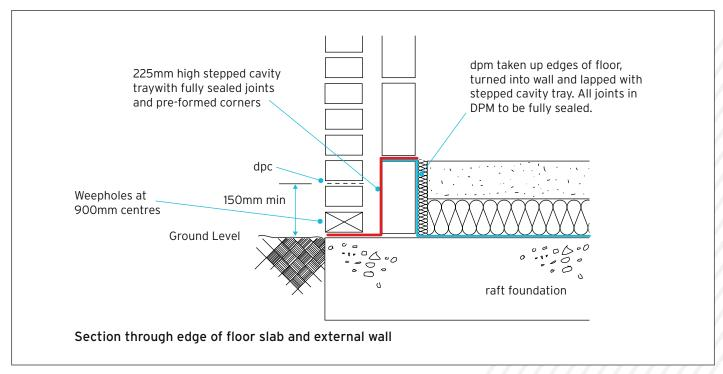
Flat slab rafts (i.e. without downward toe) should only be placed on non-frost susceptible base or soil.
