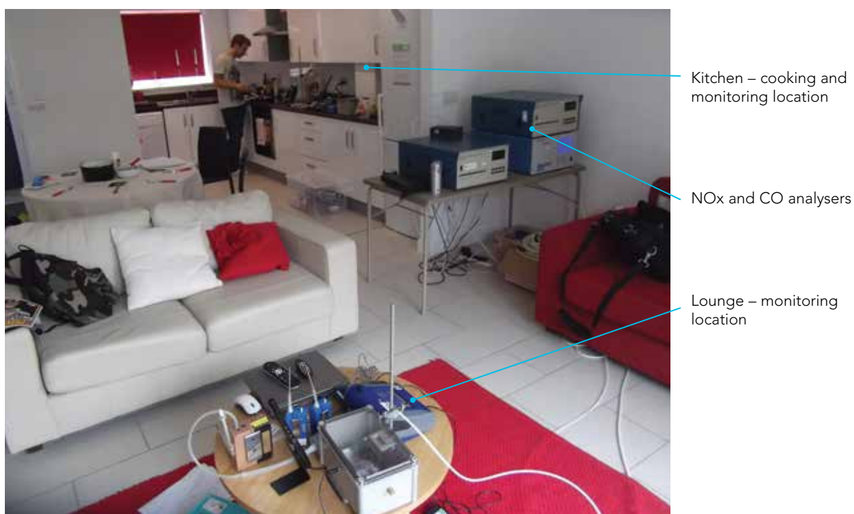
Figure 42 Overall layout of monitoring equipment in the show home
