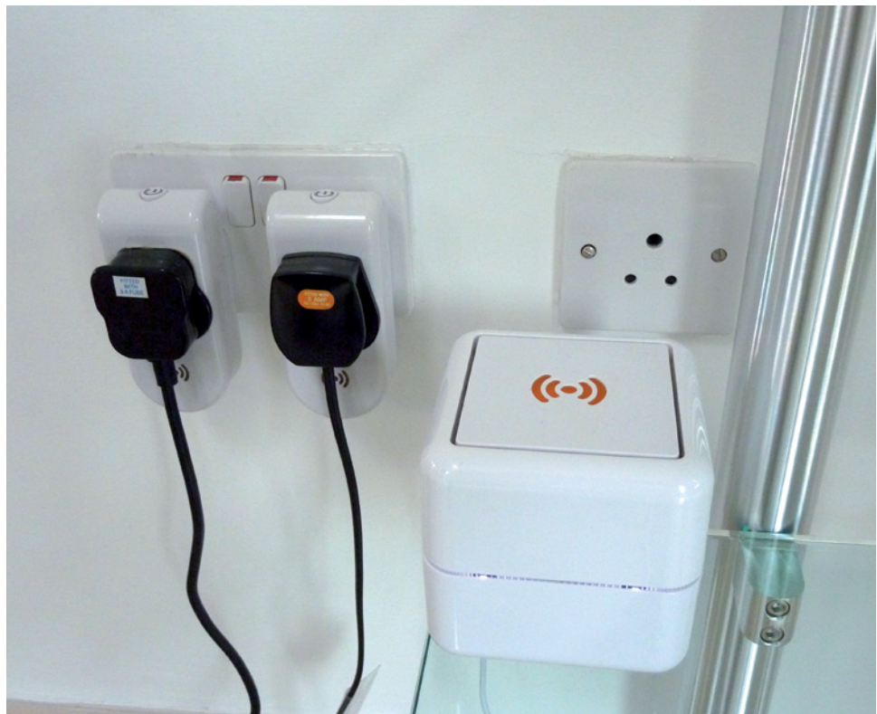
Figure 6 Example of a whole house shutdown system, showing a main control unit and plug-in appliance shutdown units. These may be integrated into the sockets themselves, or as circuits in new build applications
