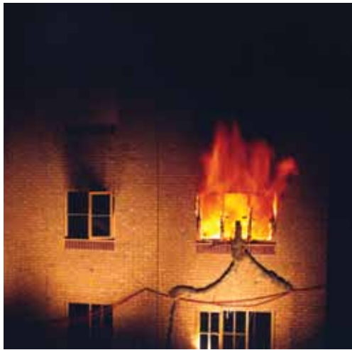
Figure 20 Compartment fire test on 2nd floor of the TF2000 building
