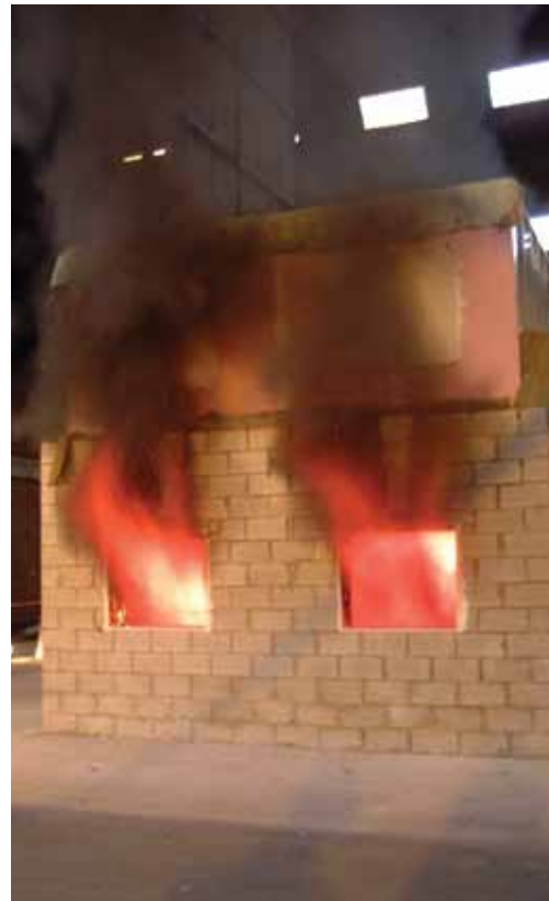
Figure 24 Fire test on light steel frame building
