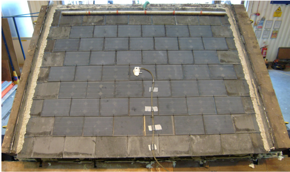
Figure 40 PV solar slates ready for testing to the MCS 012 driving rain test method.
