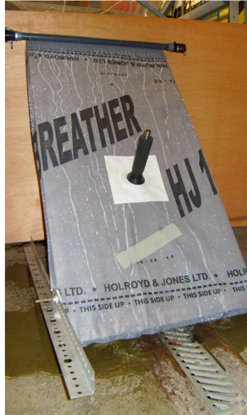
Figure 41 MCS 012 rain resistance test for underlay penetration.
