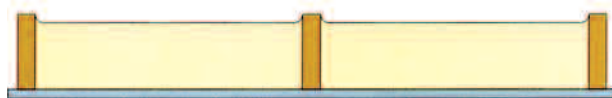
Figure 30a Roof cassette with internal structural timbers. A sheet material is used on the underside only – the foam insulation is recessed to form a ventilation gap.
