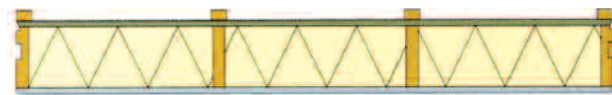
Figure 30b Roof cassette with internal structural timbers. Sheet materials are included on both faces.
