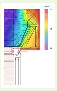
Where combination steel box lintels are commonly used considerable heat loss may occur because of the proportion of steel, the minimal and discontinuous insulation and the length of the bridge.
