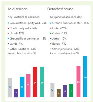
The impact of different construction junctions and the proportion of heat loss associated with each junction will both vary depending on the home type.
