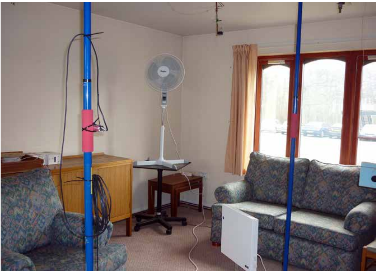
Figure 11 Typical room configuration for the BRE co-heating tests
