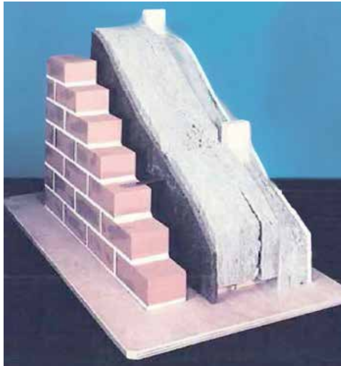
Figure A1 Model of the BRE test house wall construction
