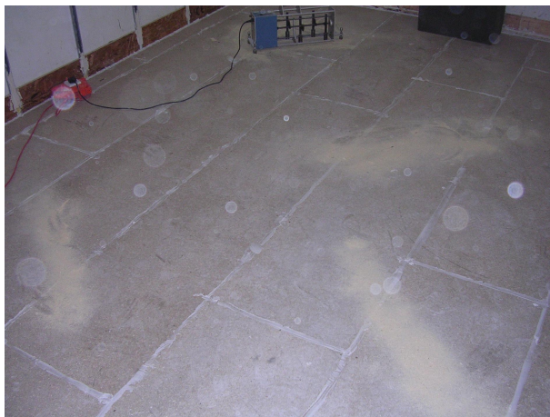
Figure 14: sawdust on timber floor for impact sound insulation measurements
