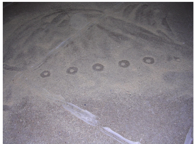
Figure 14: sawdust on timber floor for impact sound insulation measurements
