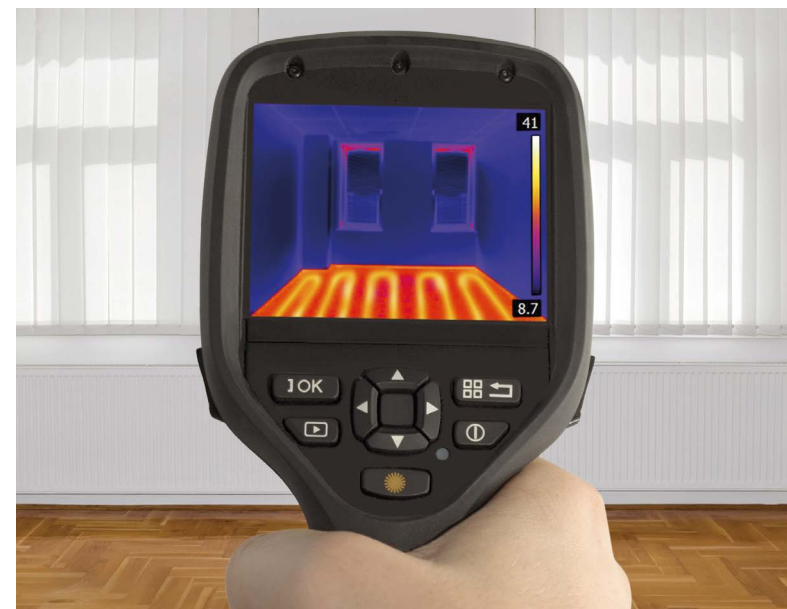
A thermal imaging camera showing underfloor heating pipe layout
