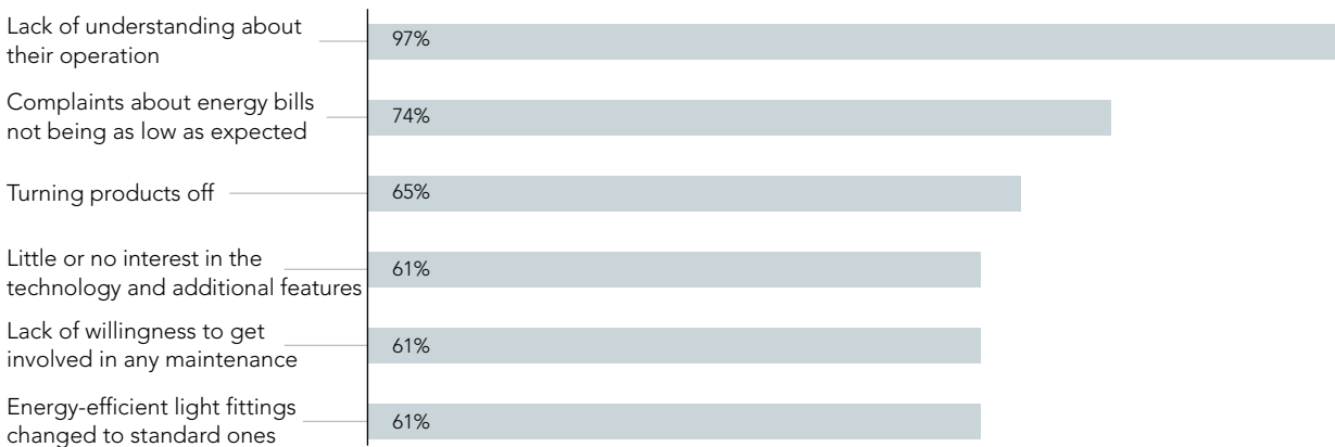
Figure 16.6 Which of these have you encountered from tenants with regard to new features and technology used to meet high Code for Sustainable Homes Levels? (Housing associations)
