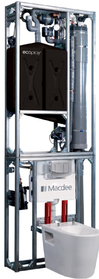
Figure 15 The Ecoplay unit allows all the water from the bath or shower to drain away and be used to flush the toilet.
