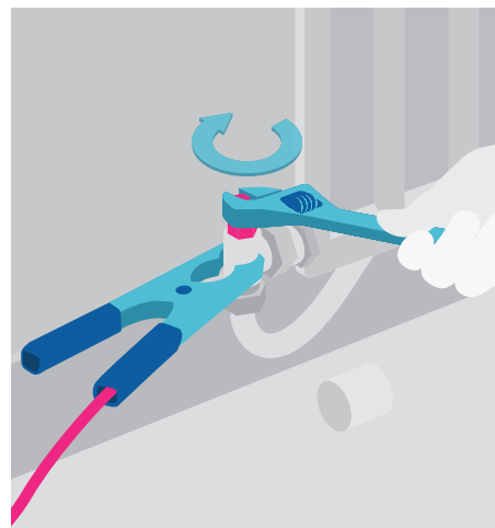
5.4 Lockshield valve adjustment
