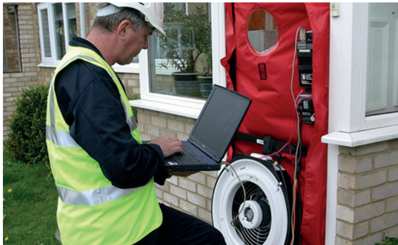
An air tightness test being carried out using a blower door kit
