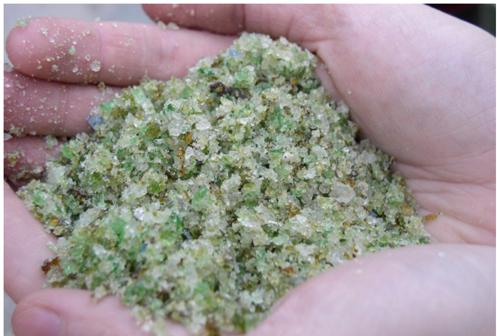
Figure 5 Bedding sand made from crushed glass
