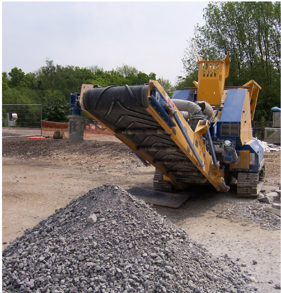
Figure 1 An in-situ crusher producing recycled concrete aggregate (RCA)
