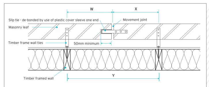
Where W & X are not more than 225mm (i.e. Y = maximum 450mm centres) no slip tie is required. Wall ties both sides of the movement joint should be spaced at maximum 300mm vertical centres.
